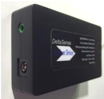
Figure 4.2.4 Green banana socket is located adjacent to the power supply receptacle.
